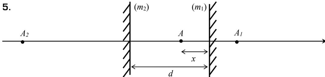
$$\overline{AA_1} = 2x ; \quad \overline{AA_2} = \overline{AA_1} + \overline{A_1A_2} = 2x - 2(d+x) = -2d ;$$
